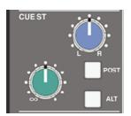
This is the channel send to the **Stereo CUE Bus**. There are separate controls for both Level and Pan, and this is normally used as a Cue audio feed for the recording artist. But this is just the beginning!
